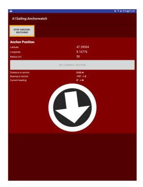
If you have to correct anchor position or radius after you already started the anchor watching process, just push the button "STOP ANCHOR WATCHING". You can now either push the button "SET CURRENT LOCATION" to overwrite latitude and longitude or you can update all parameters manually.
