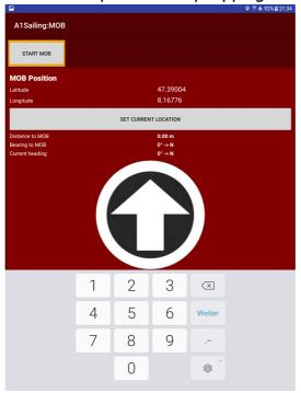
**Important notice:** Location and bearing are all based on GNSS information (no magnetic information is being used). Current heading assumes that you are currently moving. Correct bearings to MOB are only shown while you are moving (which should be normal on a sailing vessel).
